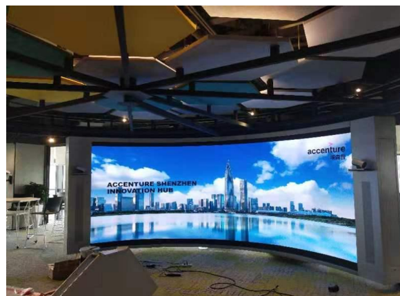
H1.56 video wall in Shenzhen Bay Science and Technology Ecological Garden
